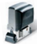
**001BX-246CU** Slide gate operator system complete with control board, chain drive, radio decoder, encoderbased movement control and obstacle detection devices. Plus, mechanical endstops for sliding gates of up to 1,320 lb. Fitted to take two 12V – 1.2 Ah batteries.
